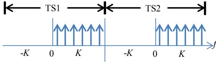
**Figure 3.** Two identical training OFDM symbols which modulate only one half of the subcarriers.
