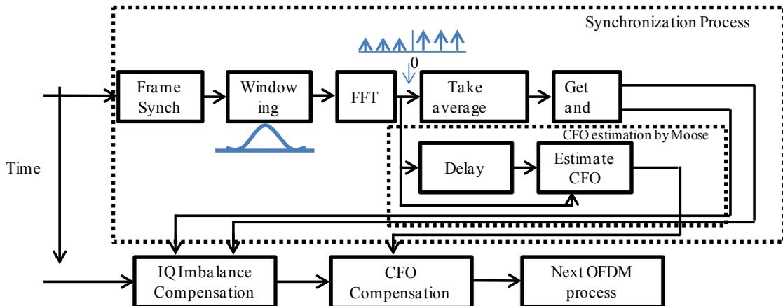
Figure 4. Simulation setup diagram.
