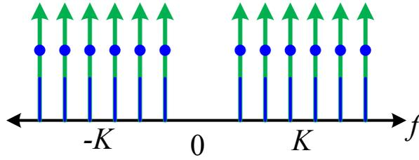
**Figure 2.** Equivalent interference image of  $K$  subcarriers due to IQ imbalance.
