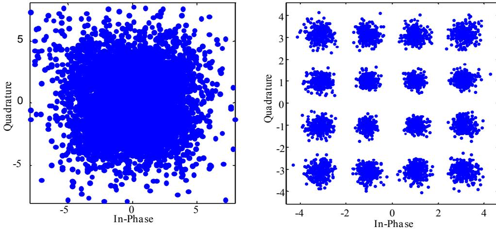
**Figure 7.** Constellation of 16-QAM; (a) before compensation of joint IQ imbalance and CFO, and (b) after compensation of joint IQ imbalance and CFO, at OSNR of 20 dB,  $15^\circ$  of phase mismatch and 15% of amplitude mismatch.
