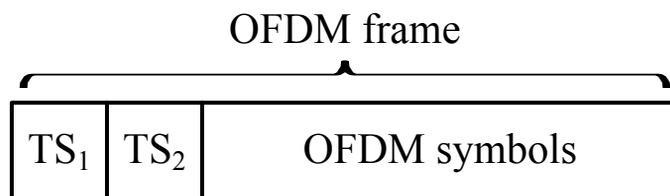
**Figure 1.** Example of OFDM frame with TS in the time domain.
