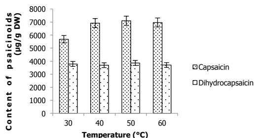
**Figure 8.** Effect of different extraction temperatures on the extraction yield of capsaicinoids in chilli pepper sample code S06
