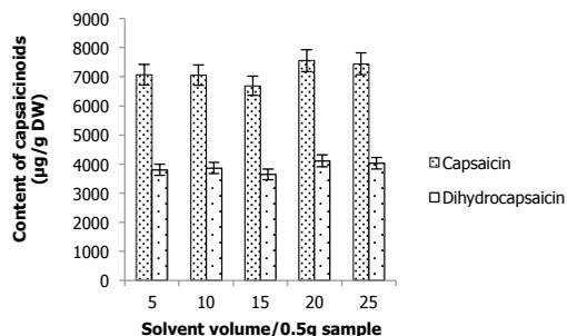
**Figure 7.** Effect of different ratios of solvent to mass on the extraction yield of capsaicinoids in chilli pepper sample code S06
