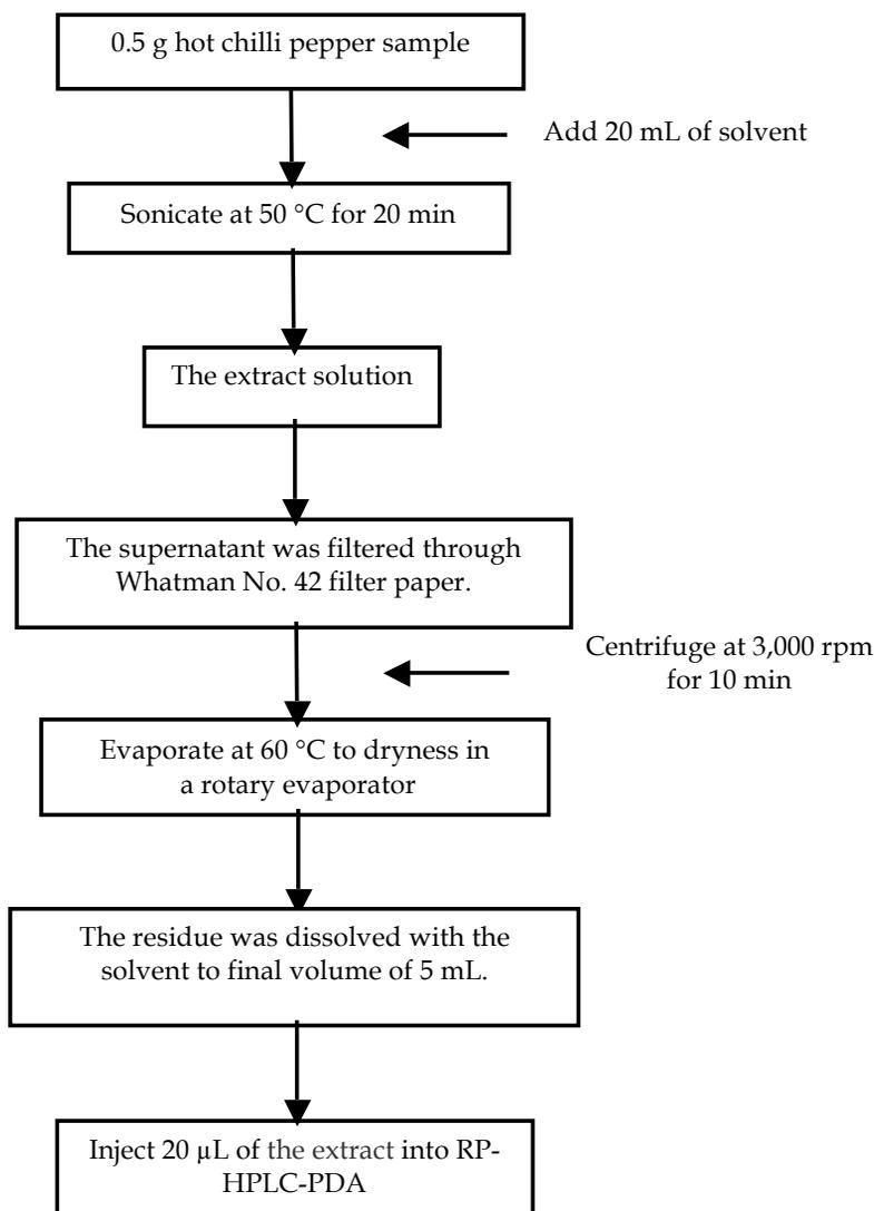
**Figure 2.** The stepwise of extraction of capsaicinoids in chilli pepper sample
