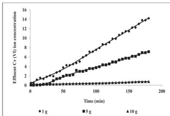
**Figure 2.** Breakthrough curves for Cr (VI) sorption onto durian peel at three different bed height on fixed bed column
