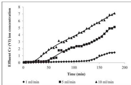
**Figure 1.** Breakthrough curves for Cr (VI) sorption onto durian peel at three different flow rates on fixed bed column
