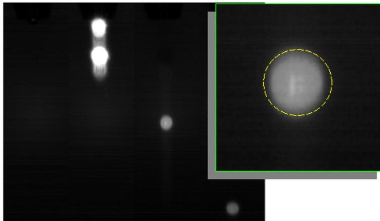
Figure 7. Molten solder ball shape after ejected from capillary.
