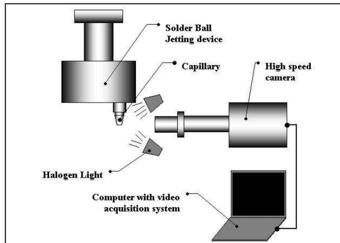
Figure 4. Schematic drawing of experiment setup.
