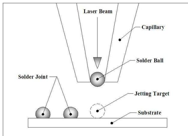
Figure 1. A solder ball was hold by capillary tip and laser energy applied to melt the solder ball.
