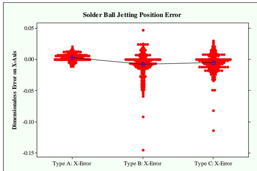
Figure 9. Comparison of solder ball jetting position error in X-direction.
