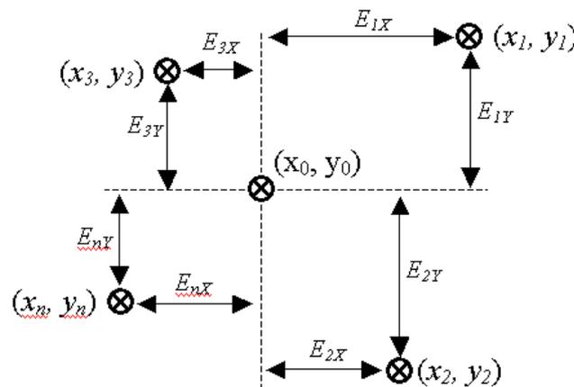
Figure 3. Solder ball jetting accuracy schematics in laser solder ball jetting process.
